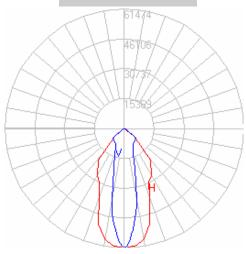
MAX CANDELA = 61474 @ 0H 0V Total Efficiency = 58% 2 Lamp, 400W, MH shown
